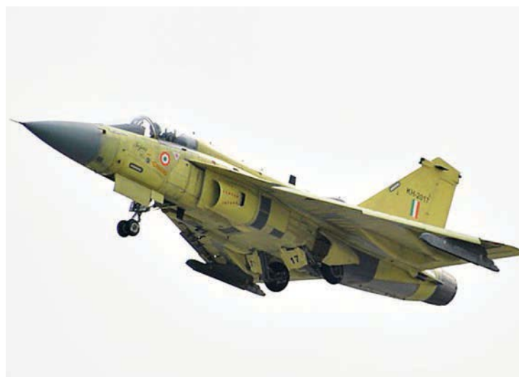
India's Tejas digital fly-by-wire light fighter features Israeli multi-mode radar, a U.S. engine and composite structures.
