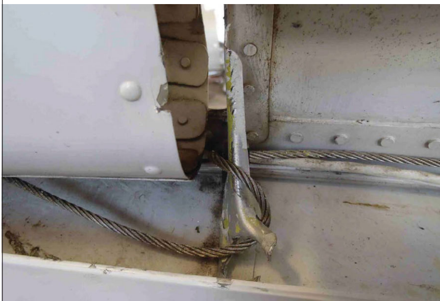
(Left wing aileron cable) The aileron remained attached at the inboard hinge, and partially attached at the outboard hinge where the tip had become bent upwards. The aileron control cable remained attached to upper portion of the control sector wheel, and had looped back through the lower balance cable rib pass-through hole.
