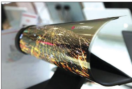
The organic layers of OLEDs are thinner, lighter and more flexible, however they are easily damaged by moisture.
