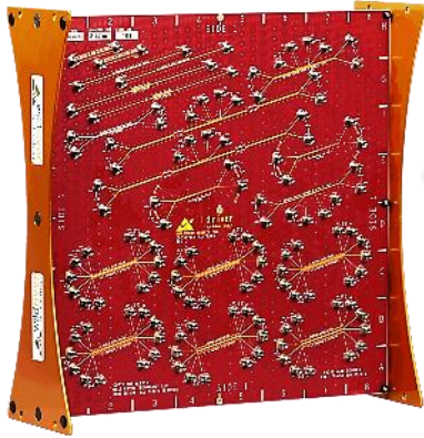
Crosstalk Noise Test vehicle, calculated RX noise as Integrated Crosstalk Noise (ICN)
