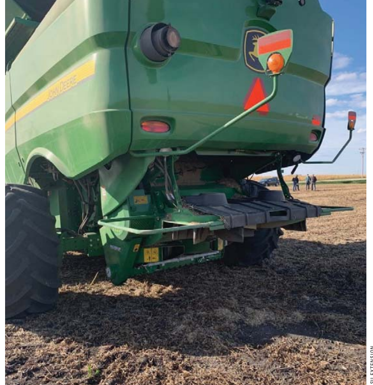
SEED DESTRUCTOR: One of the more innovative ways to control weed seeds is with a weed seed destructor. The Redekop seed destructor unit is attached to a John Deere S680 combine. The machine was recently tested in soybean fields with waterhemp infestations in central Iowa.
