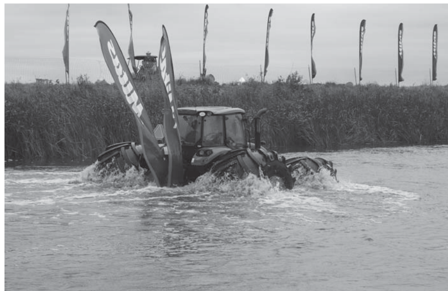
WATER WALKER: The Trelleborg/Mitas demonstration of a floating tractor at the Farm Progress Show returns for the 2022 event in Boone. The idea is to show that the right flotation matters in managing soil compactions.
