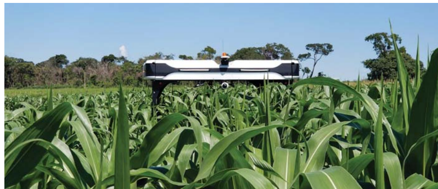
FULL-TIME DATA GATHERING: Three solar-powered autonomous vehicles from Solinftec will be at work in the autonomous demonstration area. These machines capture a range of in-season crop information to improve field management.
