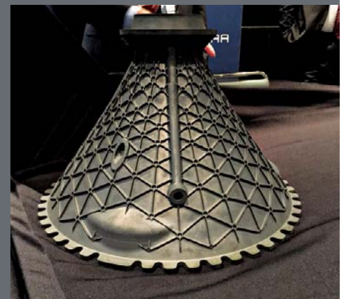
GE Aviation showed this additively manufactured test C-sump for a turboprop engine here yesterday.
