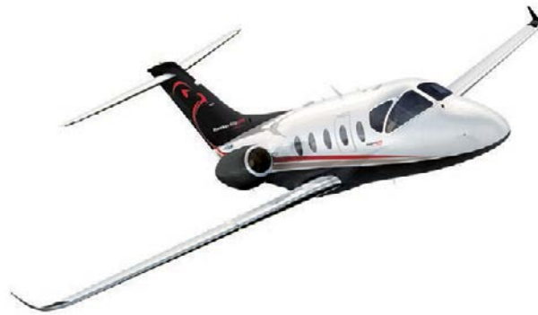
Hawker 400XPR upgrade options include winglets, Williams FJ44-4A-32 engines, and a Rockwell Collins Pro Line 21 avionics suite.
