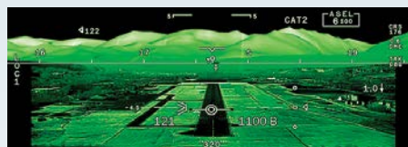
Dassault's FalconEye HUD blends database-driven terrain and thermal and low-light camera images into a single view.
