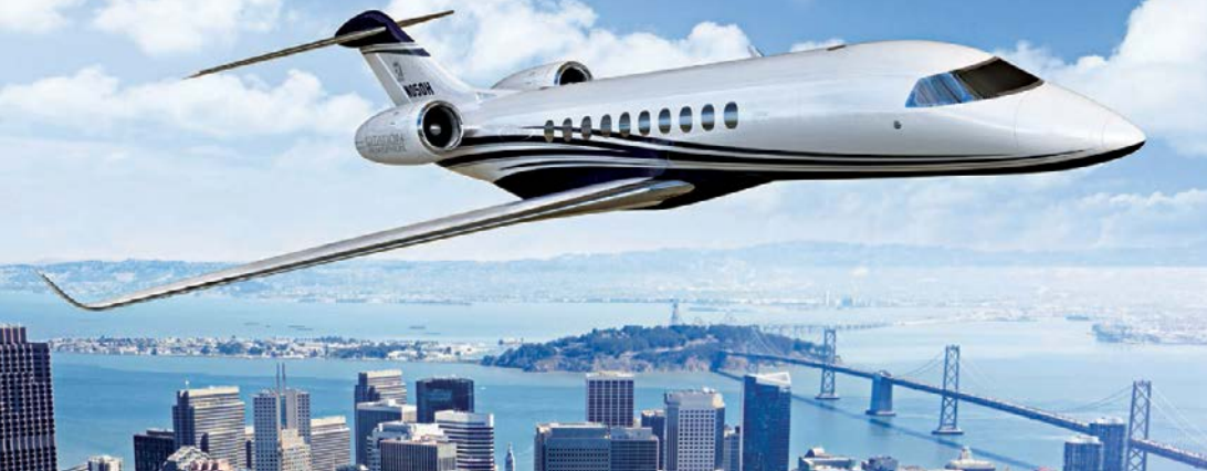
Textron Aviation's new Citation Hemisphere is to be powered by Snecma Silvercrest engines.
