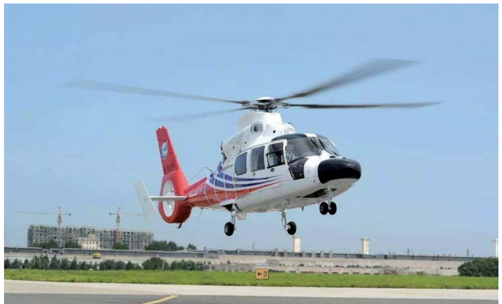
Avicopter's AC312E is powered by two Safran Helicopter Engines Arriel 2H turboshafts.
