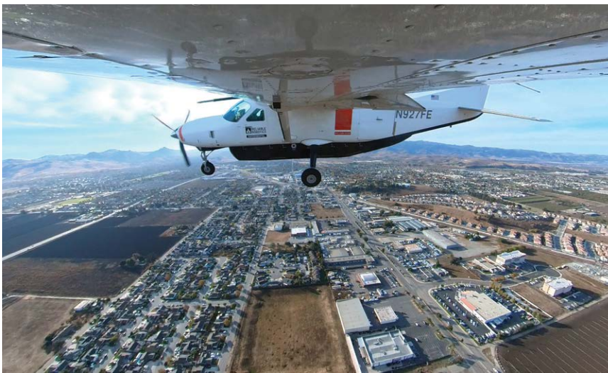
Reliable's modified Caravan first flew with no onboard pilot in November 2023.
