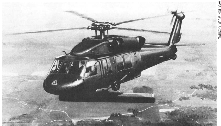
The U.S. Army wanted to adapt the Black Hawk to carry a GMTI radar developed by Motorola, as this artist's concept from the late 1970s illustrates.
