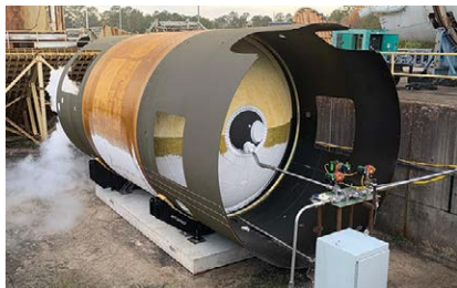
The all-composite cryogenic fuel tank at NASA Marshall Space Flight Center.
