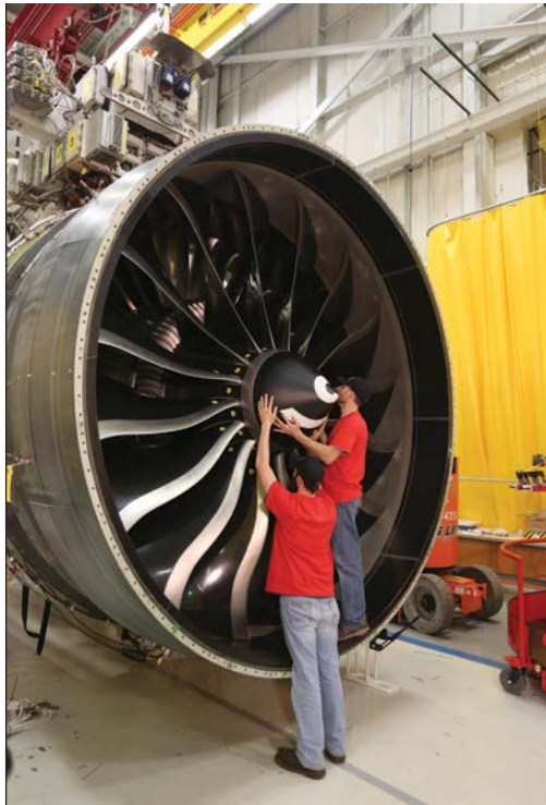
With a 134-in.-dia. fan, the GE9X is the largest turbofan ever made.
