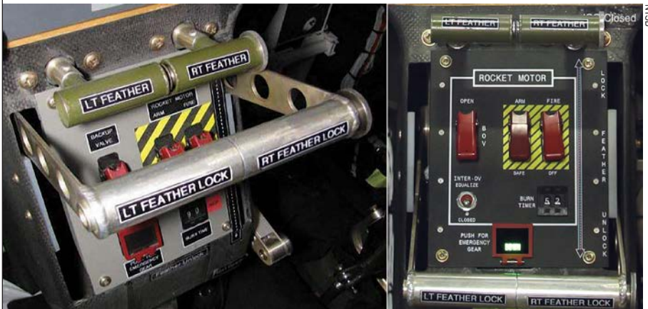
SS2's feathering tails are extended and retracted by pulling the green actuation handles mounted above the rocket motor control switches. The metallic feather locking/unlocking handle is shown (left) in the upper, locked position and (right) in the lower, unlocked position.
