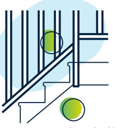
100mm spheres should not pass through
