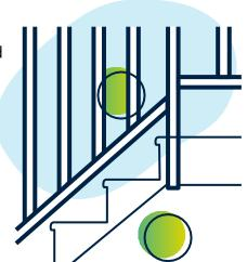
100mm spheres should not pass through
