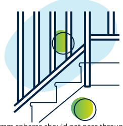
100mm spheres should not pass through
